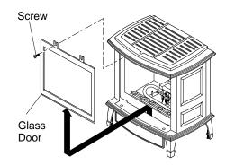
Figure 42 - Removing Glass Door from Burner System
